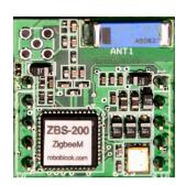
Using the module which does not require any special settings, you can directly couple it with the RXD or TXD port of user's TTL level. Communication speed is set to 9600BPS.
