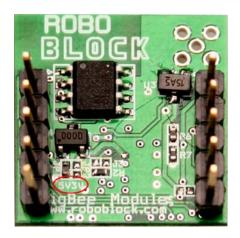
Notice: There is the sign, "0" ohm resistance that is attached in the circular part. When attached to the side of 5V, it is being operated by 5V(3.2V - 6V), and when to the side of 3V, it is working through 3V(2.8V - 3.3V). When this product is unveiled,
