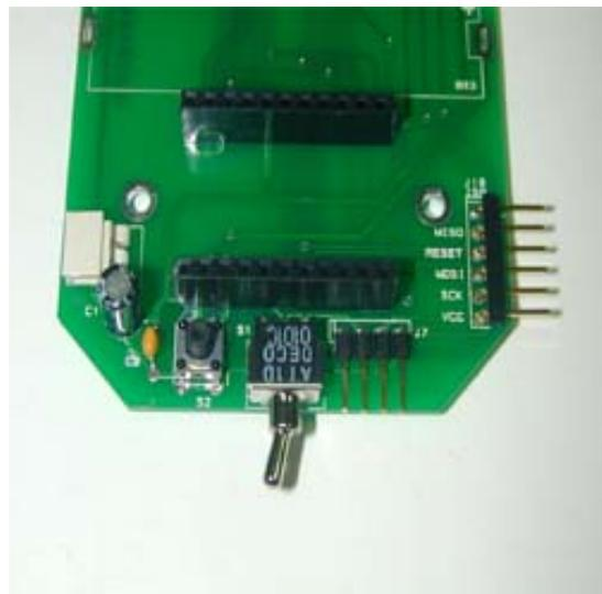
3) Solder the battery case onto BS1,2,3; the Header pin(male) onto J8 ,LEFT1, RIGHT1, MID1; resistance 330 ohm onto R1, R3 ; resistance 1K ohm onto R9, R10 ; LED onto D3, D4 ; Limit S/W into MS1,MS2.
