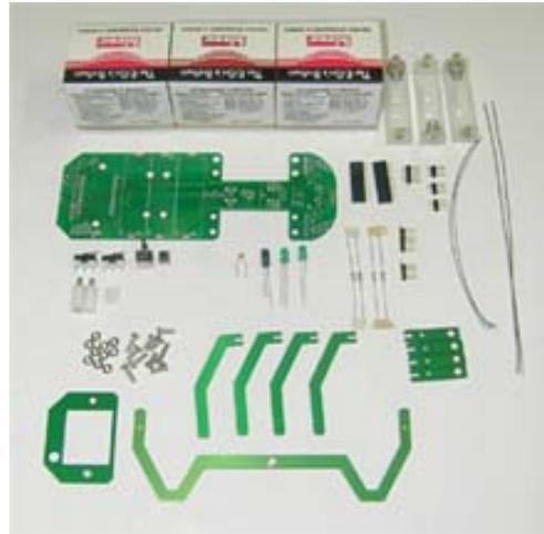
2) Solder Header pin female J4, J5, Header pin male J7, J10 (J7, 10 angle type), toggle S/W, push button S/W, 2P connector male, 10uF electrolytic condenser (white vertical line “-”), 104pF miler condenser.
